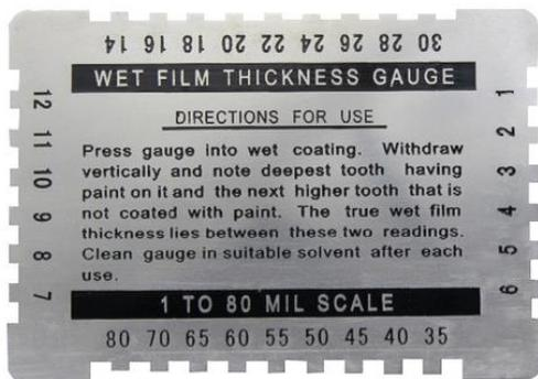
**Paint / Coatings Thickness and Uniformity** are checked by the system applicator using a wet mill gauge which when applied gives the thickness of the system prior to drying. Applicators use this as a guide based on the system’s manufactures guide. Different paint / coatings will dry to various thicknesses based on their chemical makeup and percent of solids. A simple example would be if the manufacturer recommends 3-5 mils DFT (Dry Film
